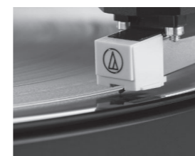
Stylus positioned over the lead-in groove just before playing
