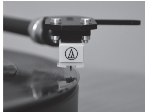
Stylus positioned over the lead-in groove just before playing
