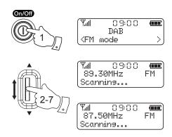
When the waveband end is reached your radio will recommence tuning from the opposite waveband end. Adjust the *Volume* control to the required setting.
