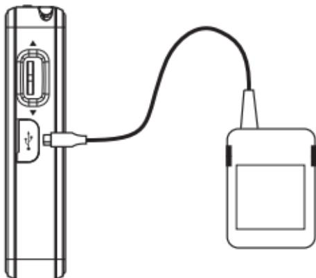
*The AC adaptor should be disconnected from the mains supply and the radio when not in use.*
