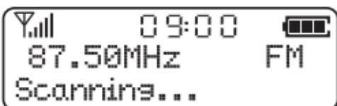
8. When the waveband end is reached your radio will recommence tuning from the opposite waveband end. Adjust the **Volume control** to the required setting.
