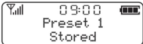
7. Press and hold the **Jog wheel** until the display shows, for example, "Preset 1 stored". The station will be stored under the chosen preset. Repeat this procedure as needed.
