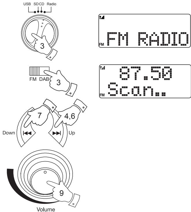
**Note:** If you find that FM reception is poor, try repositioning the Telescopic aerial. Fully extend and position vertically for optimum reception. If you find that an FM broadcast has a lot of background hiss, this may often be reduced by setting the radio into Mono reception mode for the current FM station. Please refer to the section 'Stereo/Mono setting - FM' on page 16 for further details.
