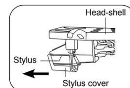
When removing the stylus cover, **do not touch the stylus**. Damage caused to the stylus by mishandling is not covered by the guarantee. When balancing the tone-arm it is important that the **stylus never contacts the turntable platter, mat or base**.
