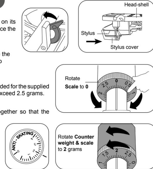
**Note:** An incorrect tracking weight can have a significant effect on the quality of the audio when playing records. If the tracking weight is set too low or too high then excessive wear to the stylus or damage to the surface of the record may be caused.
