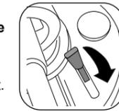
**Note:** Always use the cueing lever to lower and raise the tone-arm and stylus in order to minimise the risk of damage to either the stylus or the record's surface. **When playing records it is important to ensure that the stylus never contacts the turntable platter, mat or turntable base.** Damage caused to the stylus by mishandling is not covered by the guarantee.
