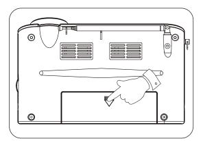
4 If the radio is not to be used for any extended period of time it is recommended that the batteries are removed from the radio.
