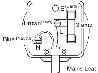
The wire coloured BLUE must be connected to the terminal marked N or coloured BLACK.
